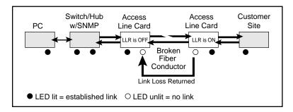
**IMPORTANT:** LLR must not be active on both ends of a configuration. If it is, the link can never be established.
